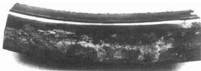
Fig. 1.51 Crevice corrosion resulting from the crevice produced between the gasket and the flange of a titanium pipe used for conveying a hot hypochlorite solution. The attacked areas are coated with a hard deposit of titanium oxides, whilst the unattacked area of metal outside the crevice remains bright
