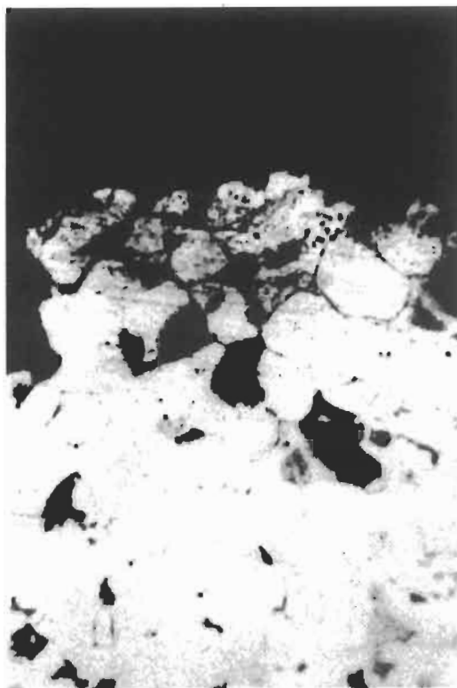
Fig. 7.52 Optical micrograph of a 5% Cr steel after service in a petrochemical plant showing typical 'metal dusting' behaviour (after Hochmann 118 )
