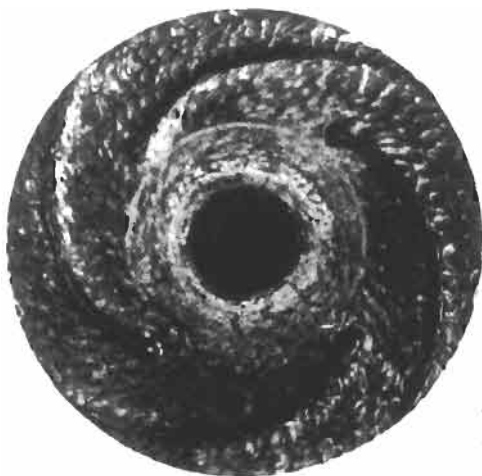
Fig. 1.61 Erosion-corrosion. Impeller fabricated from Cu-10Sn-2Zn alloy used for pumping a slurry containing 5-10% H_2SO_4 after six months' service. The blades of the impeller were extensively corroded. Note the directional form of the attack
